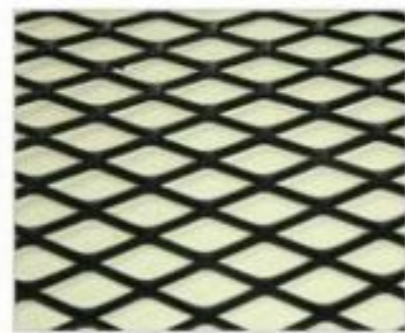
EXR 40mm - vena 3mm cal 18'' {1.2mm} resistencia 30kg/m2
