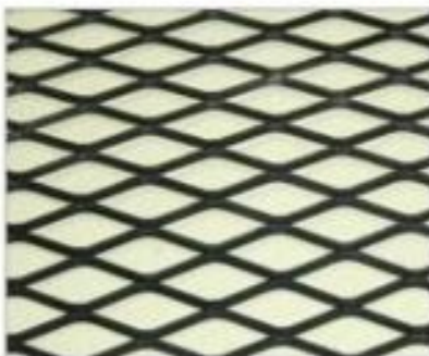
EXR 40mm - vena 3mm cal 12' {2.5mm} Resistencia 150kg/m2
